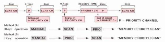
The SCAN + PRIO LED lighting evidences the correct key entry for MEMORY-PRIORITY scan operation. (See Notes 6 and 8.) To exit this operation, push the MANUAL key. During Memory-Priority scan operation, it is not necessary to enlist the Priority channel as one of Memory scan channels. The receiver will always be shifted to the Priority channel and ready to transmit as soon as the microphone is lifted off the hanger or as soon as the monitor switch is set to the "ON" position.
