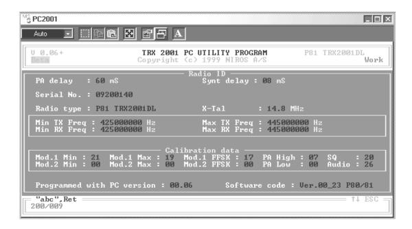
This menu provides the user with a quick overview of the basic parameters of the attached data radio, including serial number, software version, and NIROS internal calibration data.
